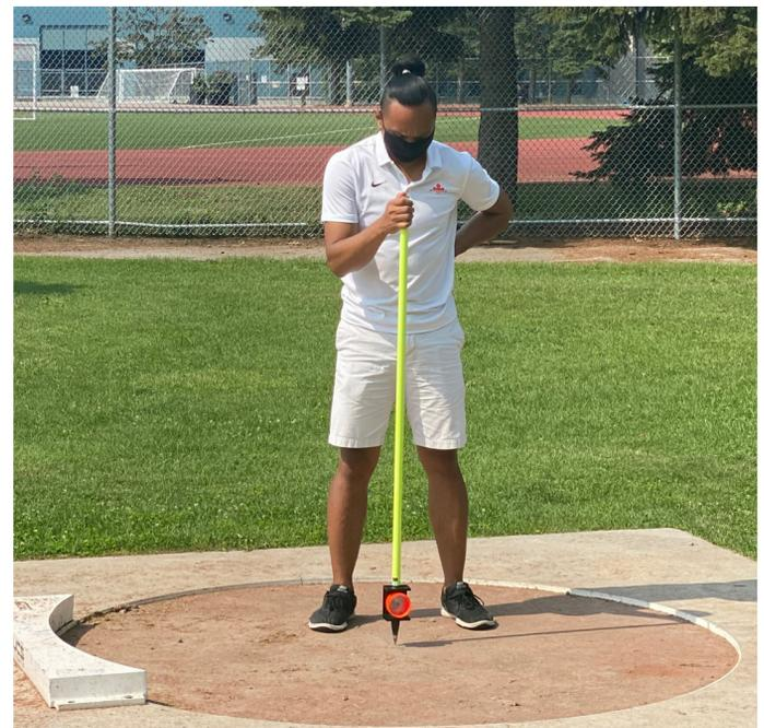
An example of a proper prism set up
